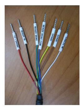
Figure 4:X-ray enable cable
